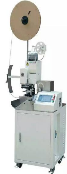
Automated Cut-To-Length, Wire Stripping, and Simple Termination
