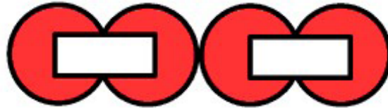
Figure 2: Diagram of a linear battery pack configuration
