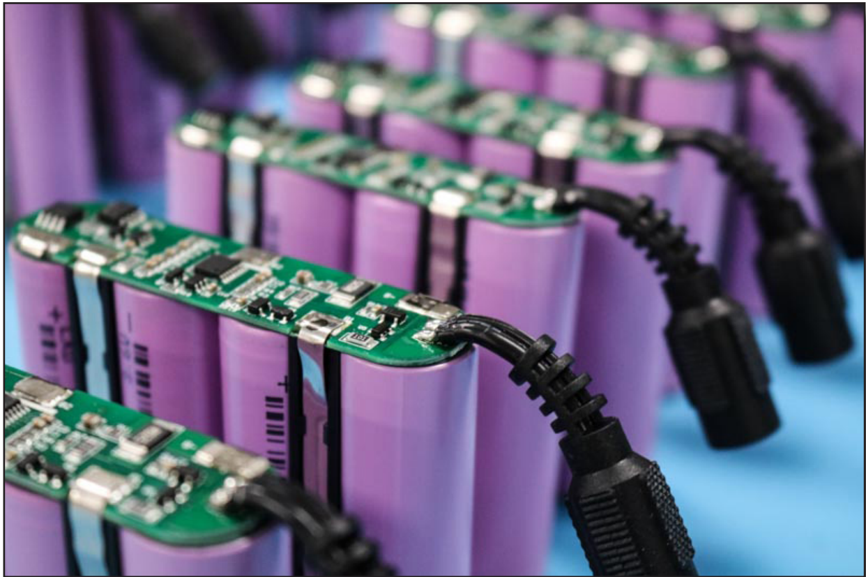
Figure 2: Lithium 4-cell pack with protection circuit.
