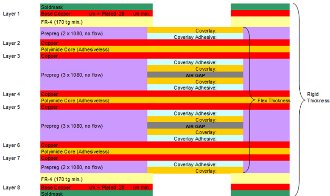
Figure 8: Example rigid-flex PCB designed with an air gap structure in the flex regions.
