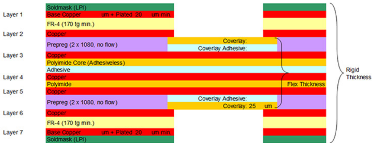
Figure 2: Example of an odd layer count rigid-flex construction.
