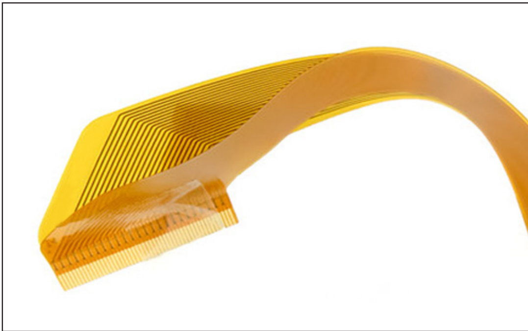
Figure 1: Example of a flexible circuit board.
