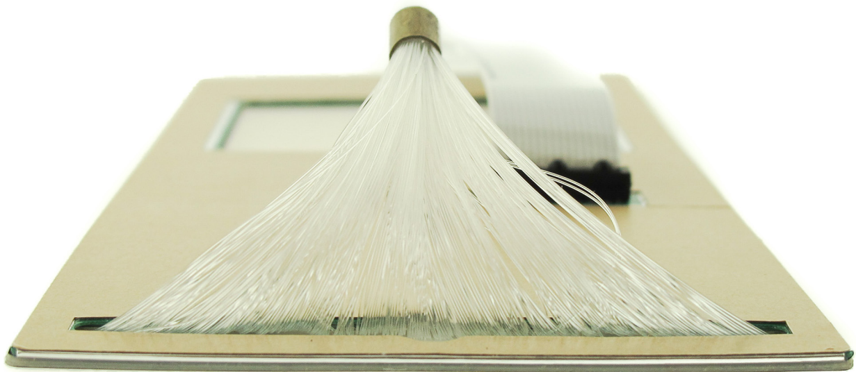
Figure 2. Fiber optic lamp at bundle end and ferrule.
