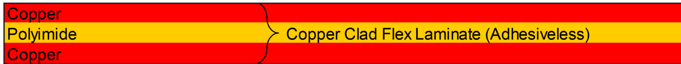
Figure 2b: An adhesiveless laminate has the copper directly attached to the polyimide core.
