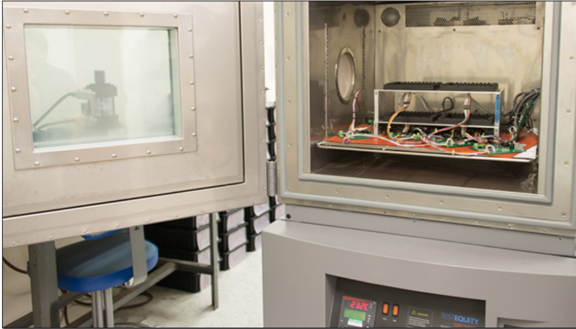
Figure 3: Example of a user interface assembly inside an environmental chamber.
