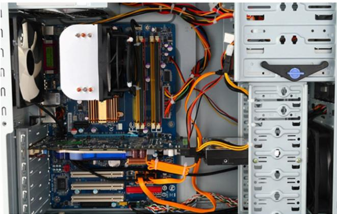
*Figure 2: Inside view of desktop computer filled with various circuit boards, connected by ribbon cables and cables assemblies.*
