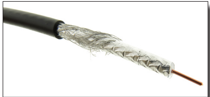
Figure 3: Example above illustrates a combination of a foil and a braid shield used to control EMI/RFI.
